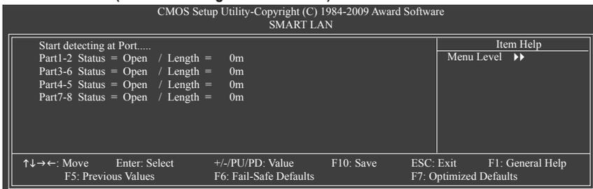
This motherboard incorporates cable diagnostic feature designed to detect the status of the attached LAN cable. This feature will detect cabling issue and report the approximate distance to the fault or short. Refer to the following information for diagnosing your LAN cable:
