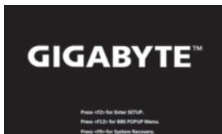
During the laptop turn on process, press and hold F9 key to launch the tool.
