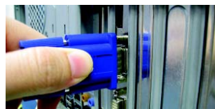
Connect a D-Sub monitor
