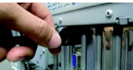
Connect an HDMI monitor
