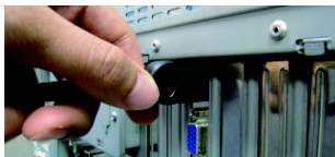
Connect a HDMI monitor
