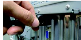
Connect an HDMI monitor
