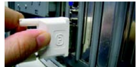
Connect a flat panel display
