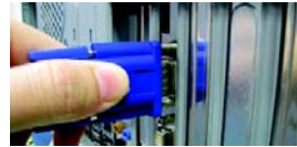
Connect a D-Sub monitor
