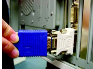
Connect a D-Sub monitor via DVI-I to D-Sub adapter
