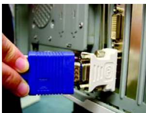
Connect a D-Sub monitor via DVI-I to D-Sub adapter
