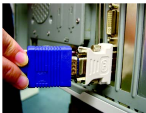
Connect a VGA monitor via DVI-I to D-sub adapter
