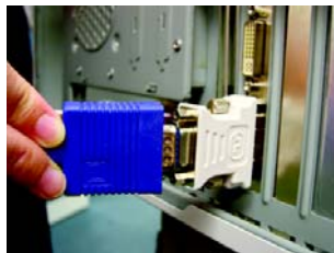
Connect a VGA monitor via DVI-I to D-sub adapter
