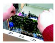
Locate the AGP slot. If necessary, remove the metal cover from this slot; then align
