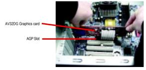
5. Replace the screw to fasten the card in place, and replace the computer cover.
