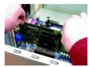
4. Locate the AGP slot. If necessary, remove the metal cover from this slot; then align your Graphics card with the AGP slot, and press it in firmly until the card is fully eated.
