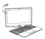
4. Lay the turned screen down into the flat position. The keyboard will be covered by the display. Use the stylus or simply touch the screen to operate U2142 as a Tablet PC.
