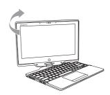
4. Lay the turned screen down into the flat position. The keyboard will be covered by the display. Use the stylus or simply touch the screen to operate U21 as a Tablet PC.
