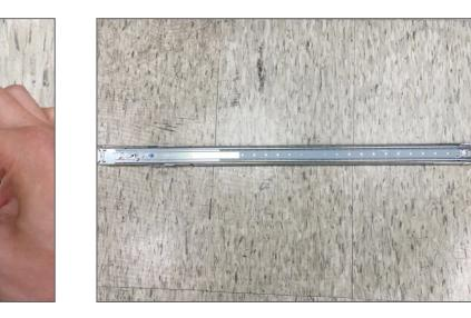
After withdrawing the front section, push back the middle section into the slide rail assembly. Push the latch and push back the middle section into the
