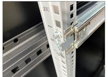
2 Unleash the metal clip to lock on the rail assembly.
