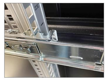
**3** The front side and rear side assembly methods are the same. Pull the metal clip and place the slide rail assembly onto the rack posts. After making sure the mounting brackets is fixed, unleash the metal clip to lock on the rail assembly. Do the same for the other slide.
