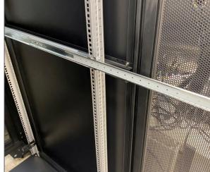
• Pull out the slide rail assembly on your rack until it stops.
