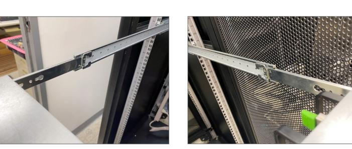
2 Align the front section of the S12 series server with the rail assembly and insert it. (NOTE: You should insert the left and right slides simultaneously to prevent any stuck during the insert process.)
