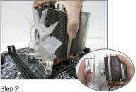
Place the cooler atop the CPU, aligning the four mounting screws with the mounting holes on the ILM. (If your cooler has a fan grill which may cause interference when you tighten the screws, remove it first and replace it after tightening the
