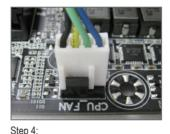
Finally, attach the power connector of the CPU cooler to the CPU fan header (CPU\_FAN) on the motherboard.
