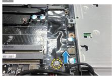
Open the rear cover and loose the screw for M.2 SSD 2
