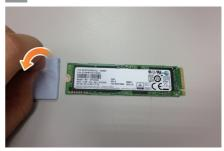
Tear the transparent film on the thermal pad
