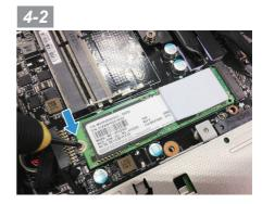
• Insert the SSD to M.2 slot and tighten the screw.
