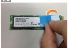
To paste the thermal pad on the top of M.2 SSD and aligned with the chip on the right side, then tear the blue film.
