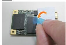
· Paste on mSATA SSD as following figure. Note the position of goldfinger and paste the thermal pad align with goldfinger
