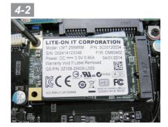
• Insert the SSD to mSATA slot and tighten the screw.
