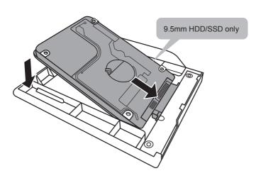
Connect the HDD or SSD pin by sliding it into the connecter.
