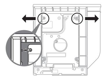
Gently push the plastic frame outwards. Slide in the HDD or SSD until it locks into place. There will be a slight click.
