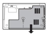
Unplug two screws and open the back cover.
