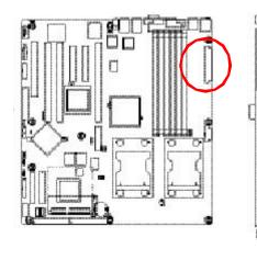
AC power cord should only be connected to your power supply unit after ATX power cable and other related devices are firmly connected to the mainboard.
