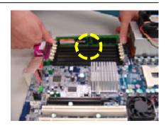
Insert the DIMM memory module vertically into the DIMM slot. Then push it down.
