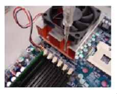
3. Fasten the heatsink supporting-base onto the CPU socket on the mainboard.
