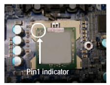
Locate Pin 1 in the socket and look for a (golden) cut edge on the CPU upper corner. Then insert the CPU into the socket.
