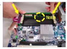
Close the plastic clip at both edges of the DIMM slots to lock the DIMM module.
