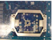
Turn the mother bord to the backside. Lock the retention module on the mother board Make sure the position of the 4 holes on the retention module match exactly the position on the motherboard.
