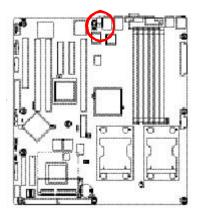
➤ To function this service switch just by pressing the white button from the back I/O.
