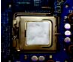
Fig.1 Please apply heatsink paste on the surface of the installed CPU.
