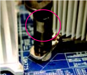
Fig. 4 Please make sure the Male and Female push pin are brought together. (for detailed installation instructions, please refer to the heatsink installation section of the user manual)
