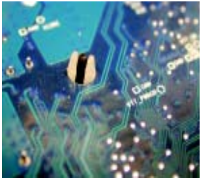
Fig. 5 Please check the back side of teh motherboard. Make sure the push pin is seated firmly as the picture shown. Installation completed.
