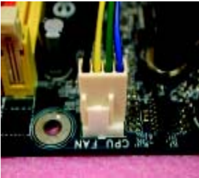
Fig. 6 Attach the power connector of the heatsink to the CPU fan header located on the motherboard.
