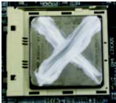
Figure 4. Application of Thermal Grease to the processor.
