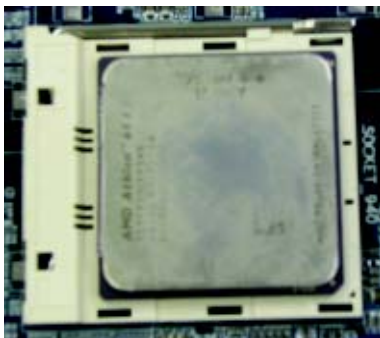
Figure 4. Application of Thermal Grease to the processor.
