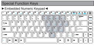
The embedded numeric keypad functions like the one on a desktop keyboard. It is indicated by small characters located on the upper left-hand corner of the keycaps.
