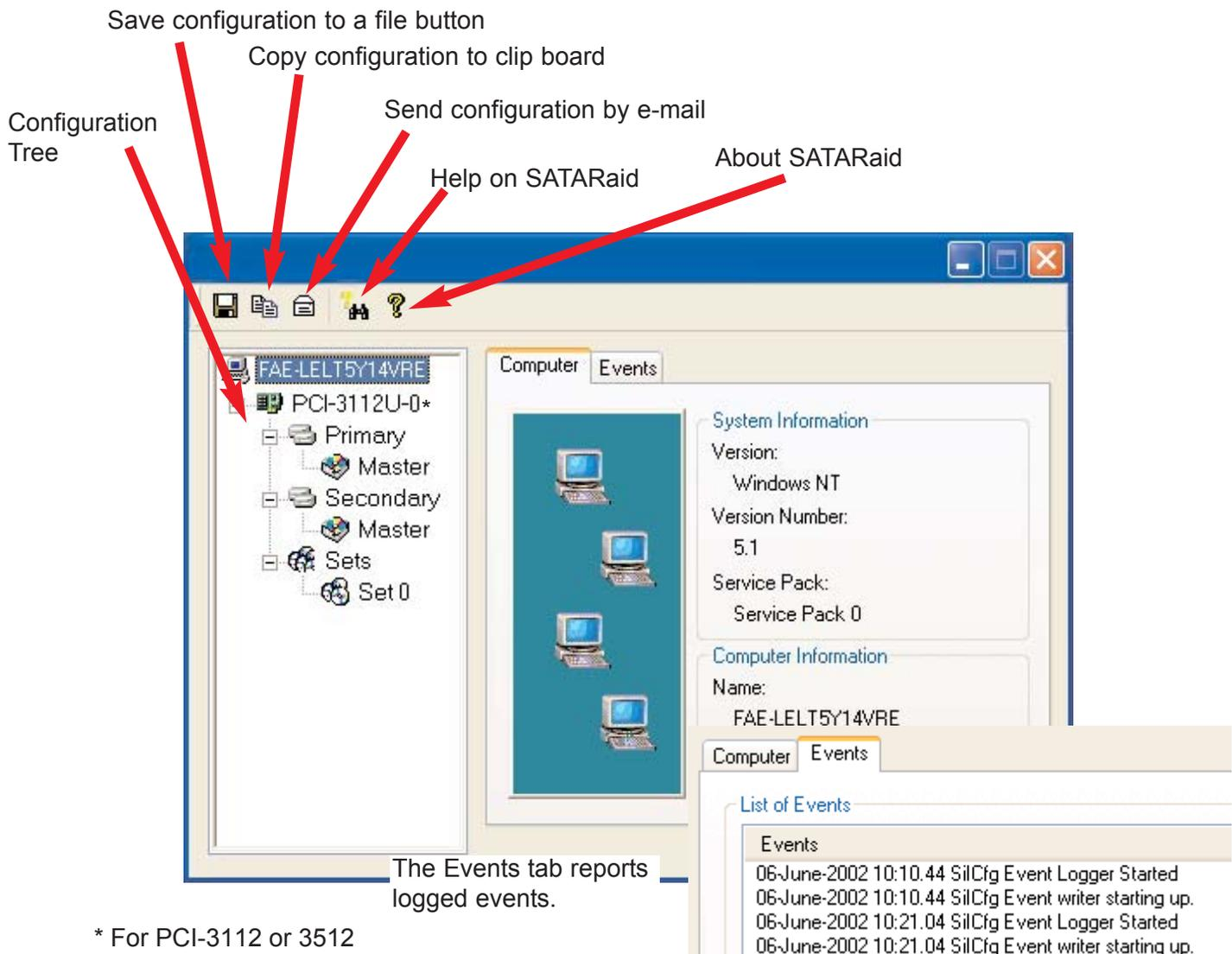
Selecting each different component in the configuration tree provides specific information for that component, such as the chip.
