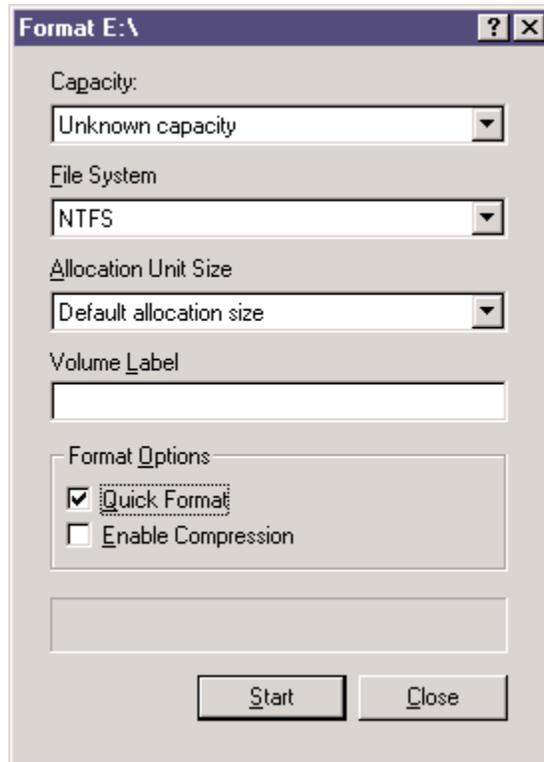
14. While **Capacity** can not be changed, make sure that **File System** has **NTFS** selected, don't change **Default Allocation Size**, and since it is the Striped Set that is being formatted, enter **Striped Set** for **Volume Label**. Make sure that **Quick Format** is selected as the **Format Option**.
