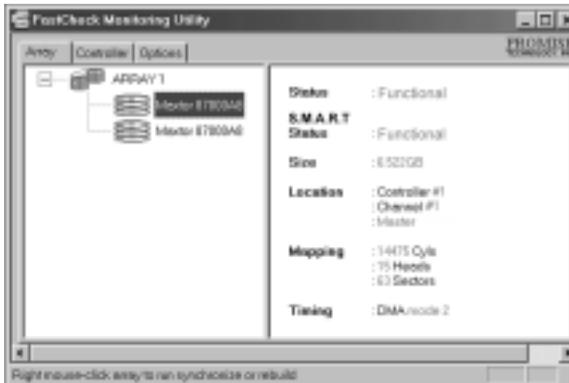
**Status** (also shown under the Array Window) can be Functional, Critical, or Offline. The meanings are shown below.
