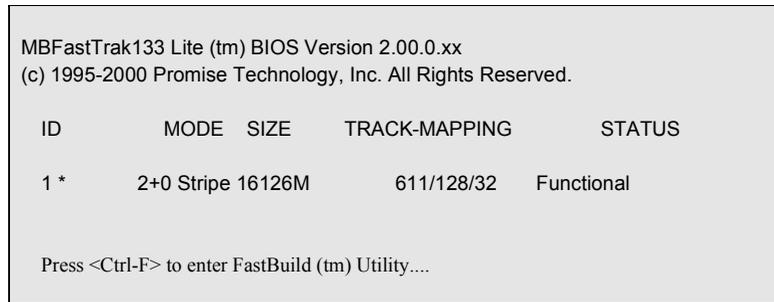
The array status consists of three possible conditions: *Functional*, *Critical*, *Offline*.
