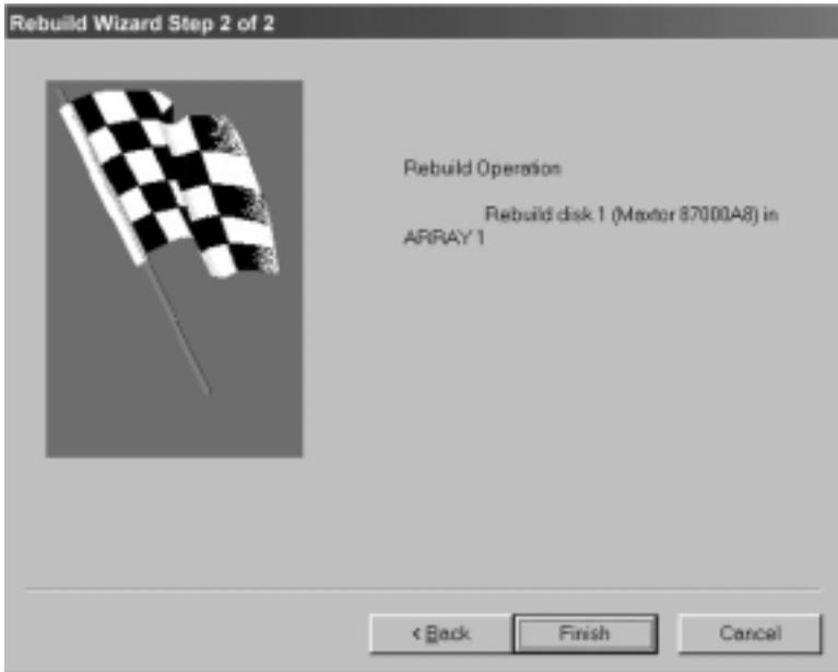
4. Rebuild Wizard Step 2 confirms the Target or "Rebuild" disk by Array # and drive ID.
