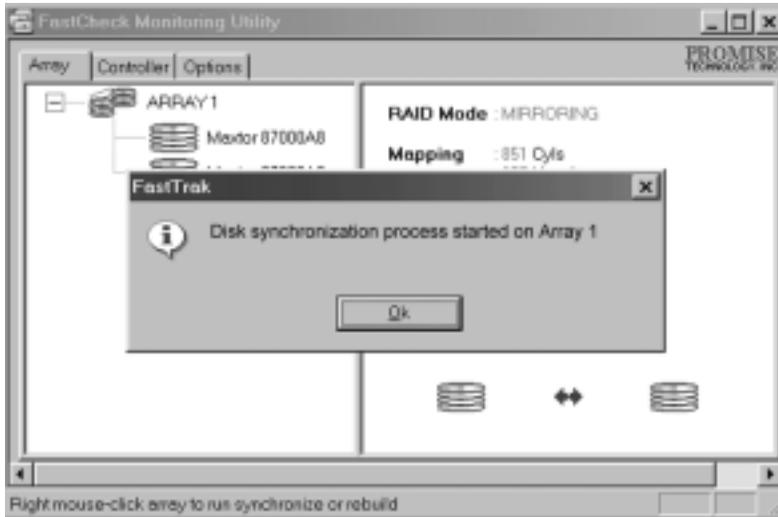
*NOTE: During Array Synchronization, users may continue to access the working array and perform normal PC functions. However, system performance will be slightly degraded and the process will take longer.*
