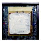
Figure 3. Application of thermal grease to the processor.
