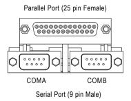
➤ This connector supports 2 standard COM ports and 1 Parallel port. Devices like printer can be connected to Parallel port; mouse and modem etc. can be connected to Serial ports.
