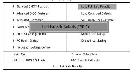
Figure 10: Load Fail-Safe Defaults
