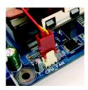
Please connect the fan heat sink power connector to the CPU\_FAN connector located on the motherboard so that the heat sink can properly function to prevent CPU overheating.
