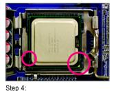
Hold the CPU with your thumb and index fingers. Align the CPU pin one marking (triangle) with the pin one corner of the CPU socket (or you may align the CPU notches with the socket alignment keys) and gently insert the CPU into position.
