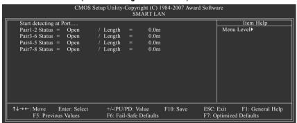
This motherboard incorporates cable diagnostic feature designed to detect the status of the attached LAN cable. This feature will detect cabling issue and report the approximate distance to the fault or short. Refer to the following information for diagnosing your LAN cable:
