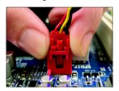
Step 1: First, attach the connector at the end of the cable to the SPDIF\_IN header on your motherboard.
