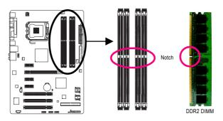
A DDR2 memory module has a notch, so it can only fit in one direction. Follow the steps below to correctly install your memory modules in the memory sockets.
