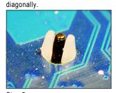
Step 5: After the installation, check the back of the motherboard. If the push pin is inserted as the picture above, the installation is complete.
