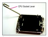
Step 1: Completely raise the CPU socket lever.
