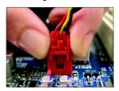
Step 1: First, attach the connector at the end of the cable to the SPDIF\_I header on your motherboard.
