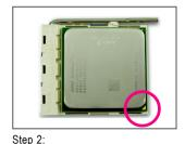
Align the CPU pin one (small triangle marking) with the triangle mark on the CPU socket and gently insert the CPU into the socket. Make sure that the CPU pins fit perfectly into their holes. Once the CPU is positioned into its socket, place one finger down on the middle of
