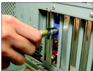
S/PDIF Coaxial Cable
