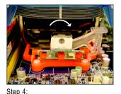
Turn the cam handle from the left side to the right side (as the picture above shows) to lock into place. (Refer to your CPU cooler installation manual for instructions on installing the cooler.)
