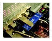
Step 4: Plug the display cable into the graphics card which on the  $PCIE\_16\_1$  slot<sup>(Note)</sup>.
