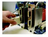
(Note) If you want to enable the SLI function, you must plug the display cable into the graphics card which on the PCIE\_16\_1 slot.
