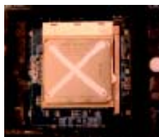
Figure 4. Application of Thermal Grease to the processor.
