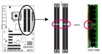
A DDR2 memory module has a notch, so it can only fit in one direction. Follow the steps below to correctly install your memory modules in the memory sockets.
