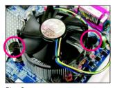
Step 3: Place the cooler atop the CPU, aligning the four push pins through the pin holes on the motherboard. Push down on the push pins diagonally.
