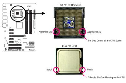
B. Follow the steps below to correctly install the CPU into the motherboard CPU socket.
