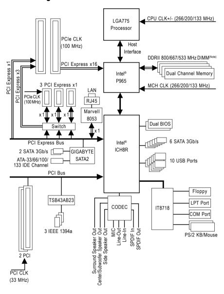
(Note) To use a DDRII 800/667 memory module on the motherboard, you must install a 1066/ 800 MHz FSB processor.
