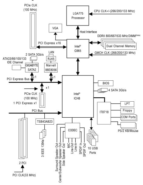
(Note) To use a DDR II 800/667 memory module on the motherboard, you must install an 1066/ 800 MHz FSB processor.
