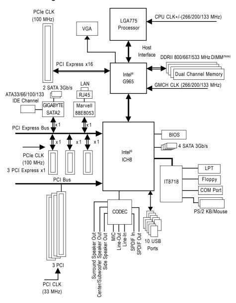
(Note) To use a DDR II 800/667 memory module on the motherboard, you must install an 800/ 1066MHz FSB processor.
