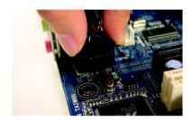
2. Secure the cable's metal bracket to the chassis back panel with a screw.
