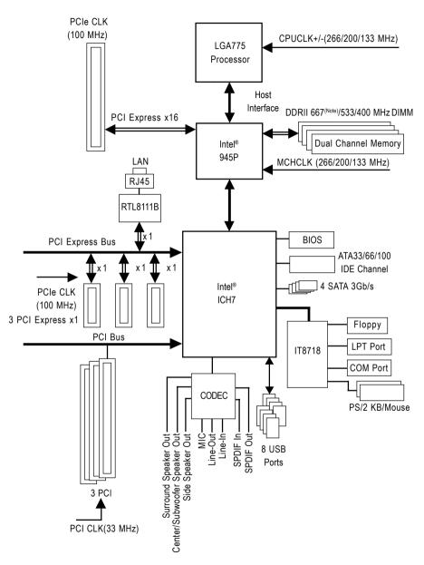
(Note) To use a DDR II 667 memory module on the motherboard, you must install an 800/1066MHz FSB processor.
