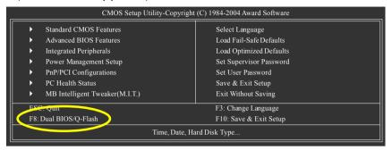
Step 2: Press F8 button on your keyboard and then Y button to enter the Dual BIOS/Q-Flash utility.
