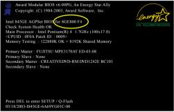
Press Del to enter BIOS menu after system reboots and "Load BIOS Optimized Defaults". See how to Load BIOS Optimized Defaults, please kindly refer to Step 6 to 7 in Part One.
