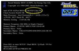
6. Press Del to enter BIOS menu after system reboots. When you are in BIOS menu, move to Load Optimized Defaults item and press Enter to load BIOS Optimized Defaults. Normally the system redetects all devices after BIOS has been upgraded. Therefore, we highly recommend reloading the BIOS defaults after BIOS has been upgraded.
