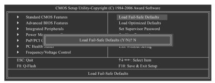
Fail-Safe defaults contain the most appropriate values of the system parameters that allow minimum system performance.
