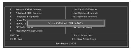
Type "Y" will quit the Setup Utility and save the user setup value to RTC CMOS. Type "N" will return to Setup Utility.
