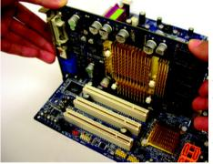
When installing the graphics card, push down on the top edge of the card until it is fully inserted into the PCI Express x16 slot. Make sure the card is securely seated in the slot and does not rock.
