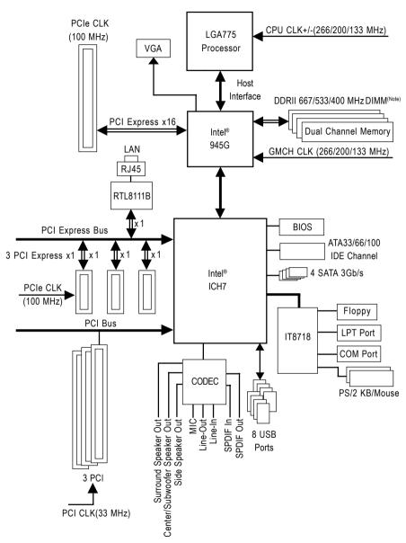
(Note) To use a DDRII 667 memory module on the motherboard, you must install a 1066/800 MHz FSB processor.
