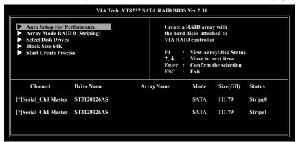
If you select a RAID 0 array, the block size of the array can also be selected. Use the arrow key to select Block Size and press **Enter**, then select a block size from the popup menu. The block size can be 4KB to 64KB.
