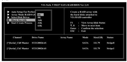
Use the arrow key to select **Start Create Process** and press **Enter**. A warning message will appear [**The data on the selected disks will be destroied. Continue? (Y/N)], press <b>Y** to finish the creation, or press **N** to cancel the creation.
