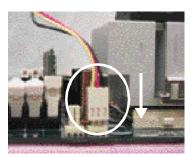
Make sure the CPU fan is plugged to the CPU fan connector, than install complete.
