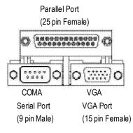
➤ This connector supports 1 standard COM port, 1 Parallel port and 1 VGA port. Device like printer can be connected to Parallel port, mouse and modem etc can be connected to Serial ports.
