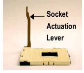
2. Pull the rod to the 90-degree directly.
