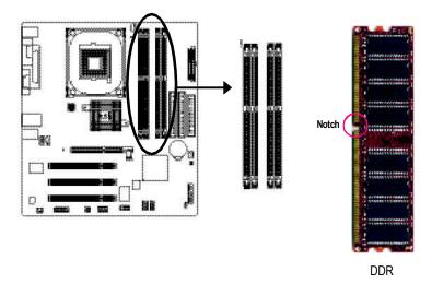
GA-8TRS300M supports the Dual Channel Technology. After operating the Dual Channel Technology, the bandwidth of Memory Bus will add double up to 6.4GB/s.
