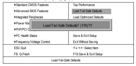
Figure 10: Load Fail-Safe Defaults
